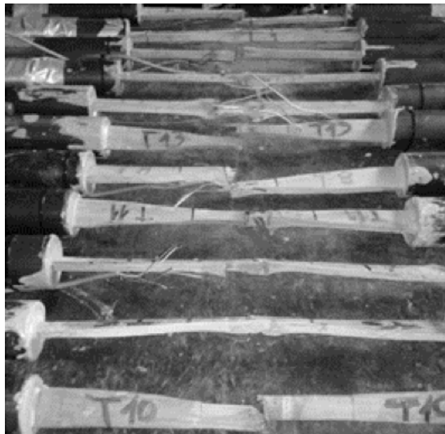
Image 3. Tension specimens after the test (Córdoba, 2014)
