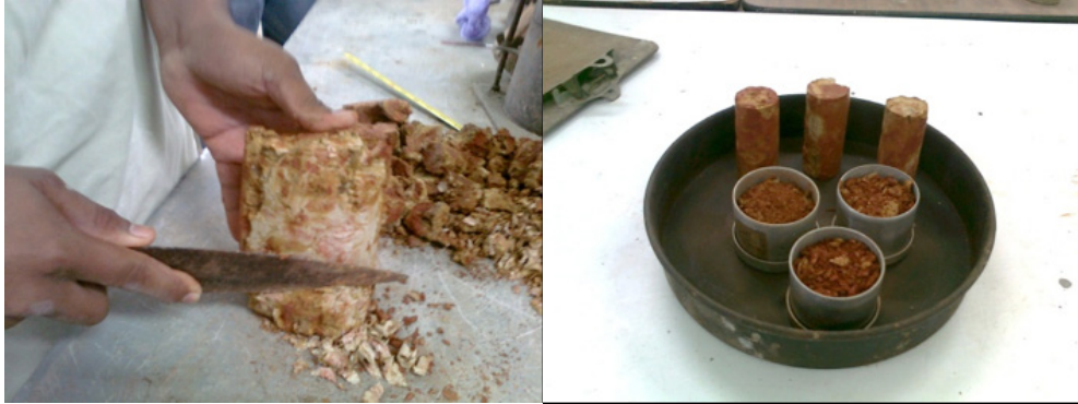
Image 2. Processing of specimens for the triaxial test
