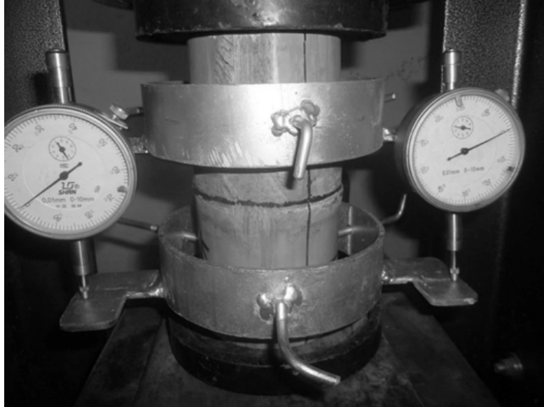
Image 1. Strain measurement system in compression test
