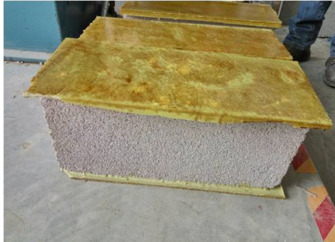
Image 3. Individual pieces with sulfur pitch
