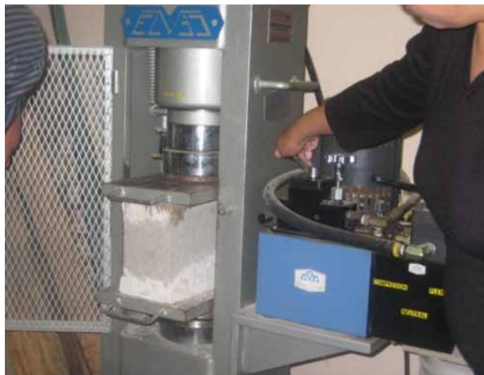
Image 14. Compression test. Source: Own elaboration
