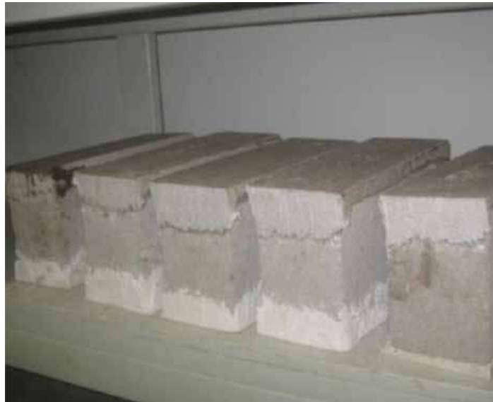
Image 13. Pitching of the mortar blocks. Source: Own elaboration
