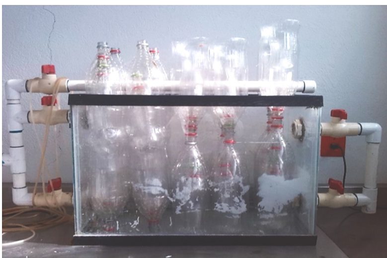
Figure 1. Aerobic reactor with PET bottles as medium of support.
