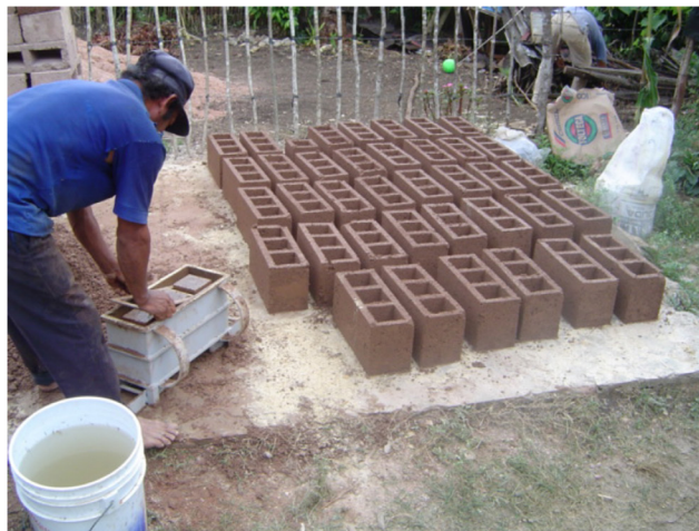
Image 6. Hollow block pieces with three cells
