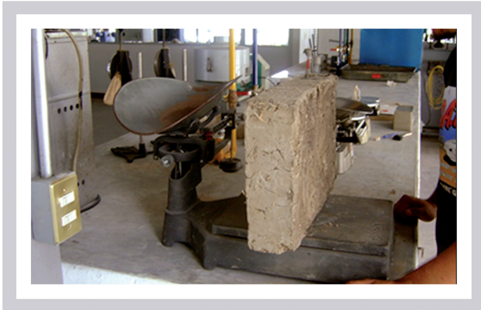
Figure 2. Obtaining the weight of each of the parts of tested adobe (Ovando Ruíz de la Cruz and Castellanos, 2010)
