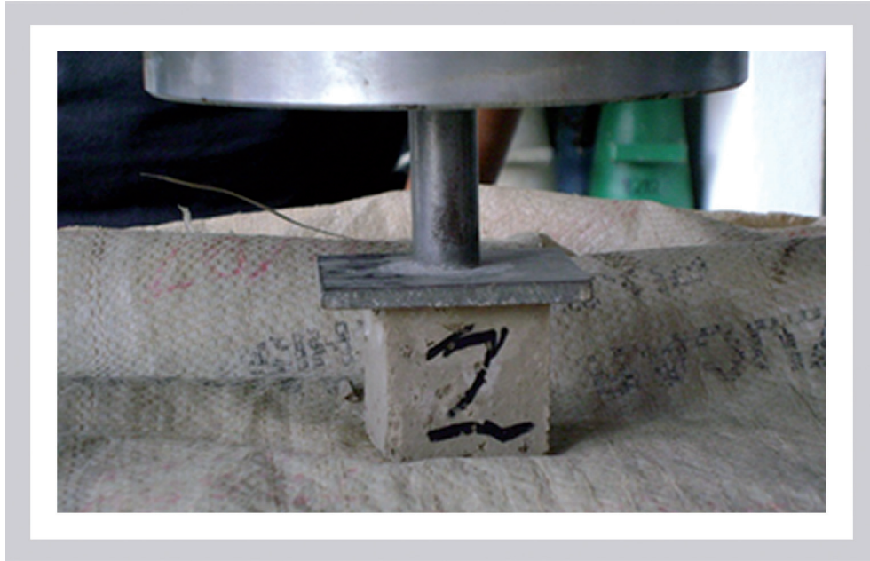
Figure 6. Compression test on clay mortar specimens (Ovando de la Cruz y Ruíz Castellanos, 2010)
